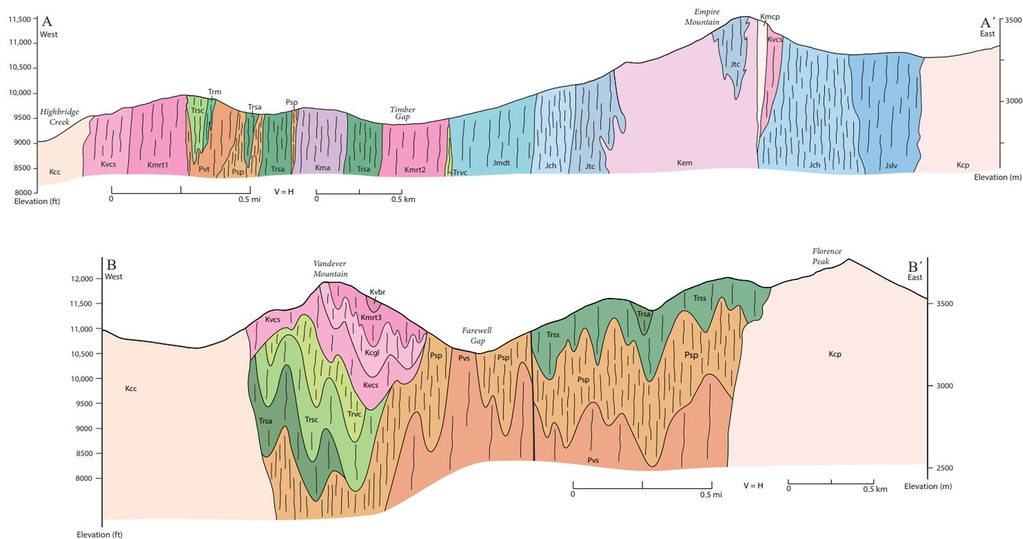
**Figure 4.** Cross sections of the Mineral King pendant, California, USA. Quaternary surficial deposits are omitted. Thin, wavy lines indicate approximate orientation of foliation. See geologic map (Fig. 3) for locations and geologic unit descriptions.
