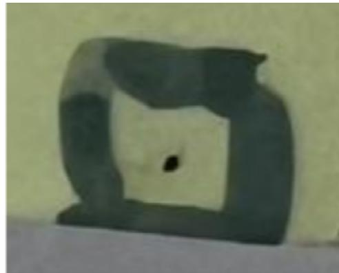
**Figure 7:** Photograph of  $\text{Cs}_3\text{Bi}_2\text{Br}_9:\text{Mn}$  film after being illuminated by a 405 nm laser for 30 minutes.
